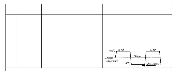
Note: When there are questions concerning, measurement shall be made after 24 2hrs of recovery under the standard condition.
